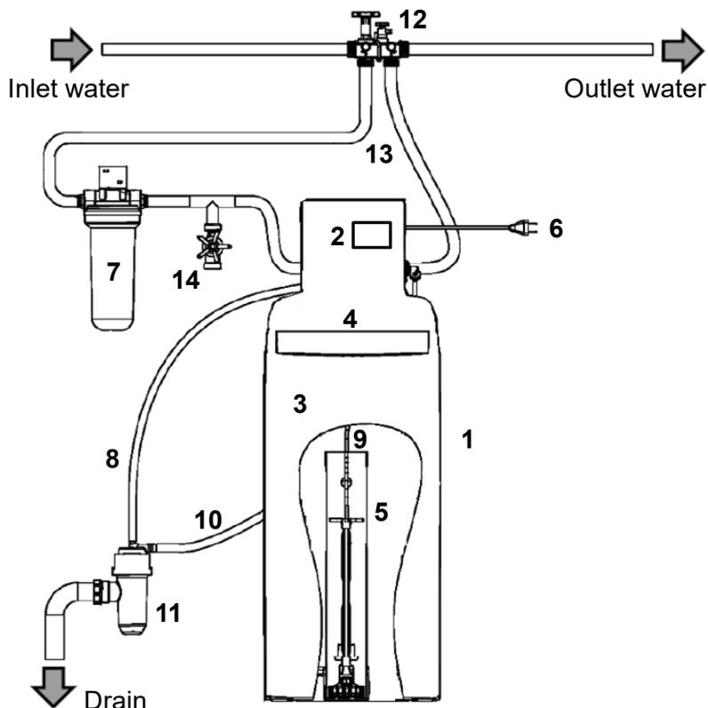
It is under the installer's responsibility to make sure that the installation does not generate any water hammer which could damage the proper work of the softener. It is highly recommended to connect the device with flexible hoses.
